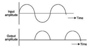
The main supply voltage is given to the transformer which will increase or decrease the voltage and give to the diode. In most of the cases we will decrease the supply voltage by using the step down transformer here also the output of the step down transformer will be in AC. This decreased AC voltage is given to the diode which is connected serial to the secondary winding of the transformer, diode is electronic component which will
